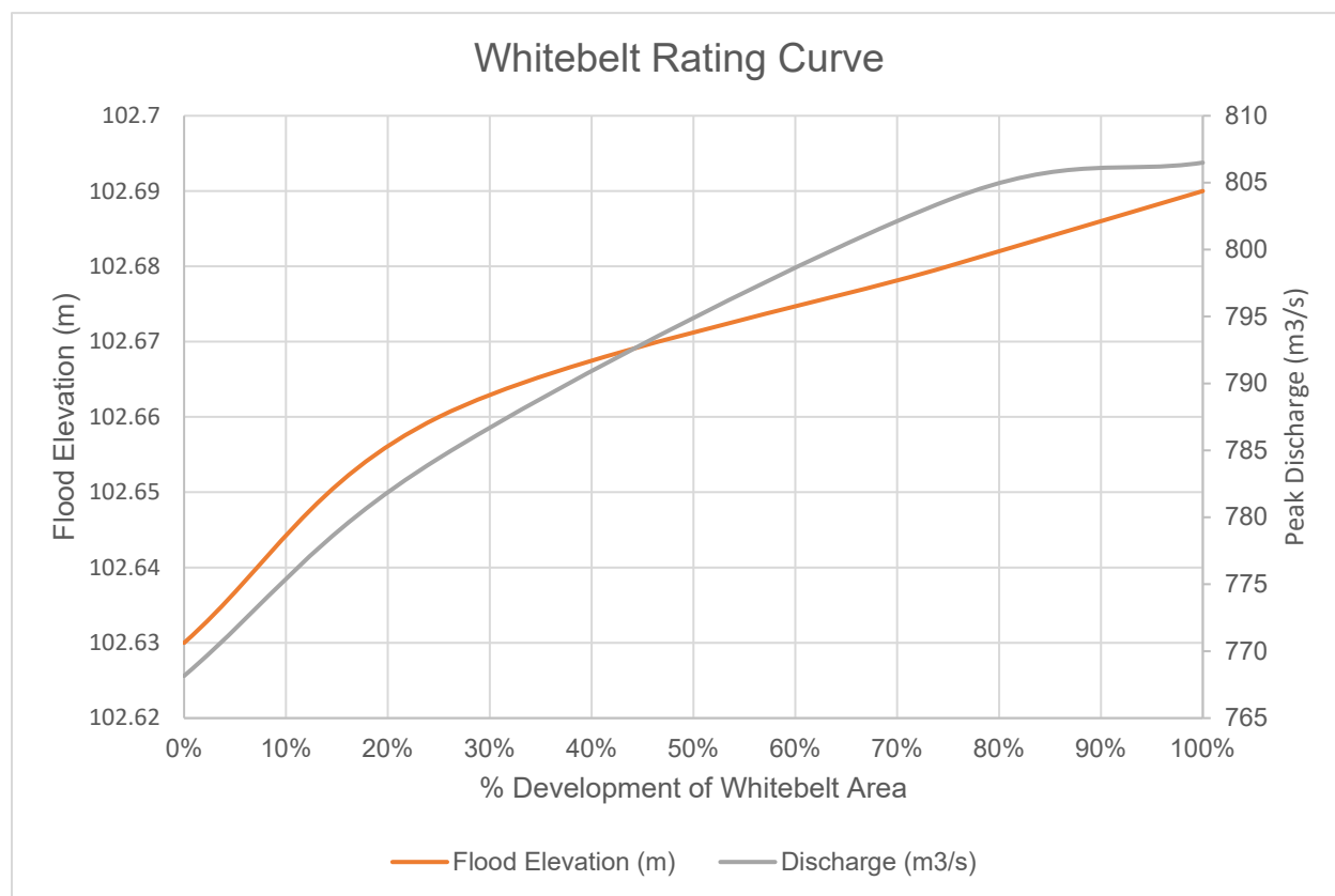
FIGURE 4.11A: WHITEBELT RATING CURVE FOR THE CPR BRIDGE
