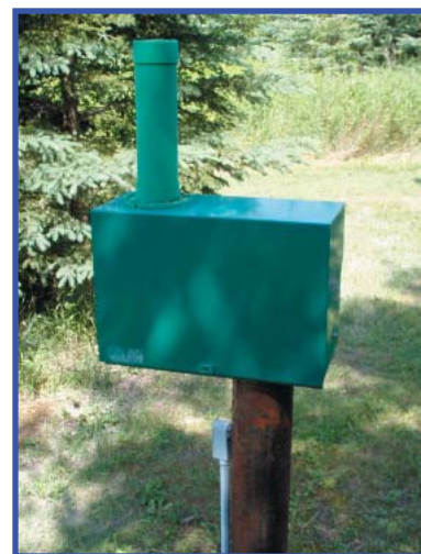
Groundwater monitoring well at Enniskillen C.A.
