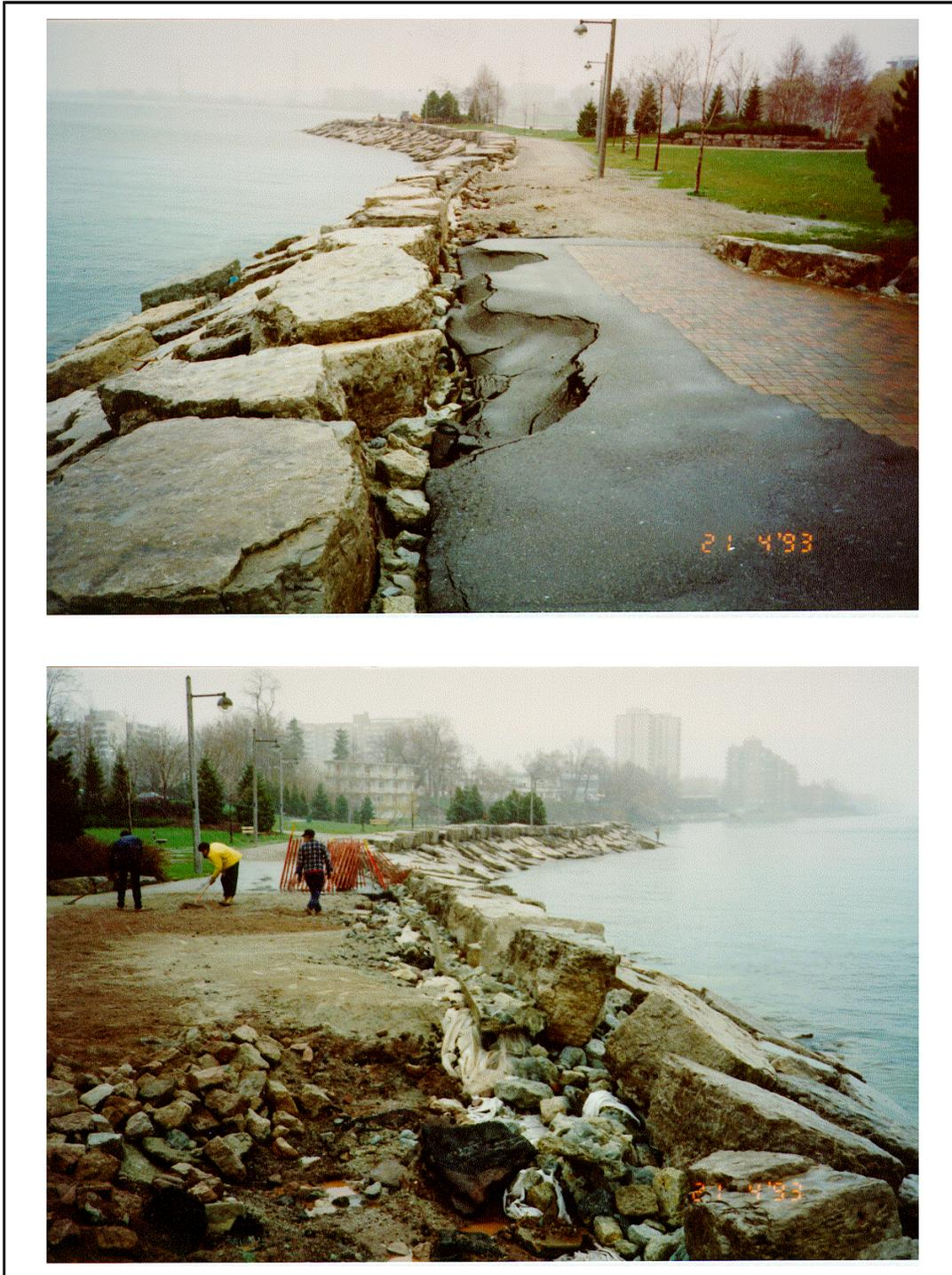
In an attempt to determine the rip-rap layer stability for angular shaped stones when subjected to overtopping flow, the rip-rap layer median stone size  $D_{50}$  was correlated to the overtopping unit discharge at failure,  $q_f$  ( $q_f$  should be a momentary discharge per characteristic wave and not the time-averaged discharge,  $Q$ ) and found to be:
