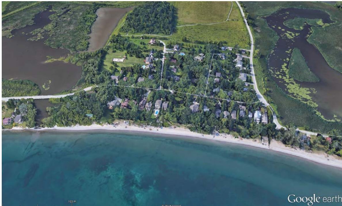
Figure 2.9: Shoreline backed by Cove Road in centre of image, showing larger setbacks for houses compared to adjacent shorelines along Cedar Crest Beach Road and West Beach Road
