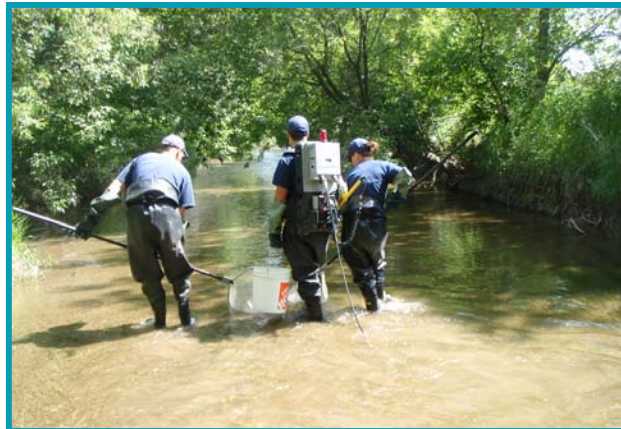
Electrofishing equipment is used to gather fisheries samples. Above a backpack unit is used in a creek and below a special boat is used in larger bodies of water.
