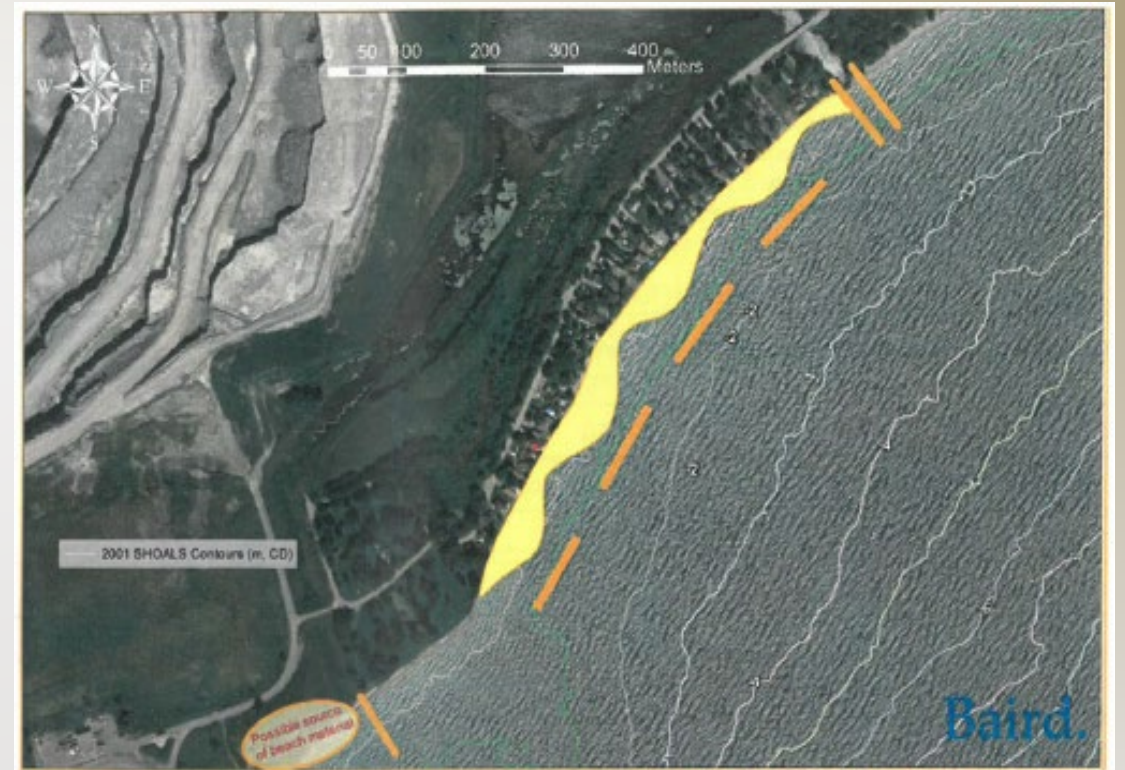
Figure 3.3: Concept 3 – Sand and cobble beach with offshore breakwaters and jetties at Westside Creek, flood channel
