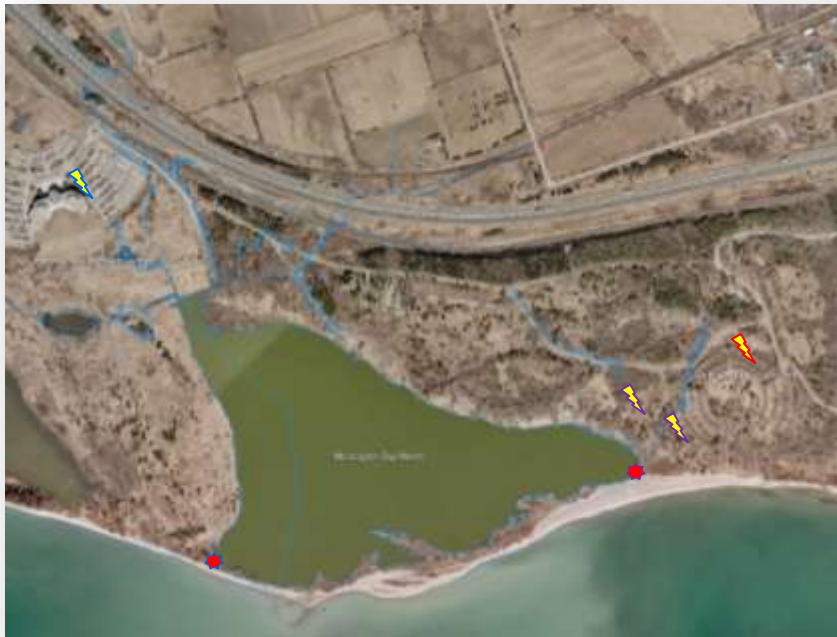
FIGURE 14: POTENTIAL HYDRO CONNECTION POINTS AND LOCATIONS FOR A PERMANENT ELECTRIC PUMP HOUSE AT MCLAUGHLIN BAY.
