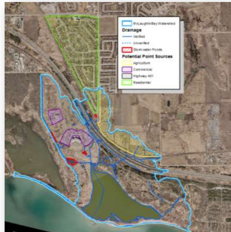
FIGURE 20: MCLAUGHLIN BAY WATERSHED WITH STORMWATER PONDS, POTENTIAL POINT SOURCES FOR CONTAMINANTS, AND CREEKS.
