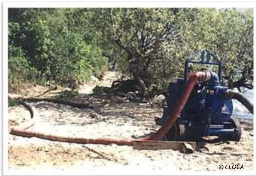
FIGURE 3: PORTABLE DIESEL PUMP.
