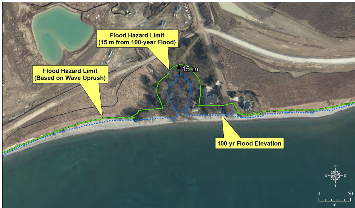
Figure 5.5 Sample of the Flood Hazard Limit with Runup Calculations and the 15 m Setback
