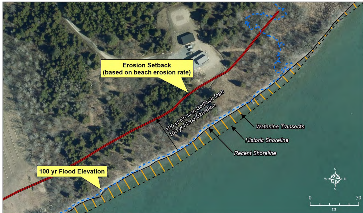
Figure 5.3 Erosion Hazard Setback Methodology for Beach Shorelines
